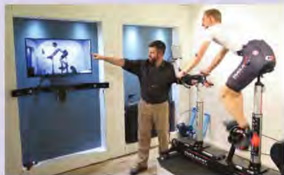
Figure 9.4 Modern bike fitting is an interactive process incorporating data from a variety of sources such as three-dimensional motion analysis, shoe and saddle pressure distribution, and pedal force application
