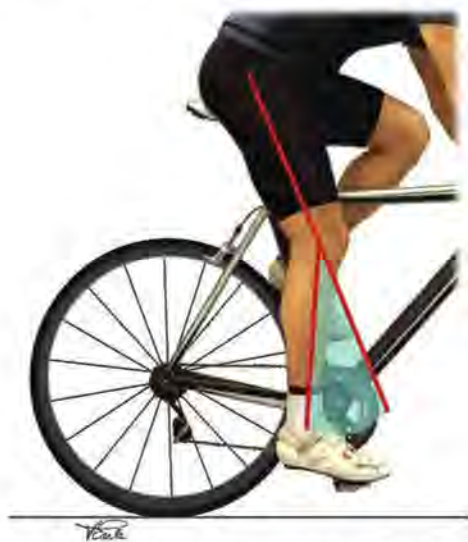
Figure 9.1 Maximum knee extension is a key bike fitting parameter, which typically ranges from 35–40° among professional riders. Patellofemoral joint contact pressures may be minimised by selecting a higher saddle position, with maximum knee extension between 30° and 35°.
