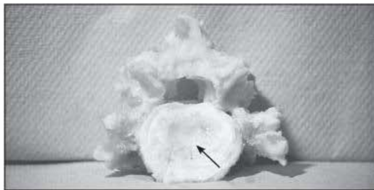
Figure 4.7 Stellate-patterned end-plate fracture (indicated with arrow) occurs as the nucleus is pressurized under compressive load, which causes it to bulge the end plate, imparting tensile stresses.
