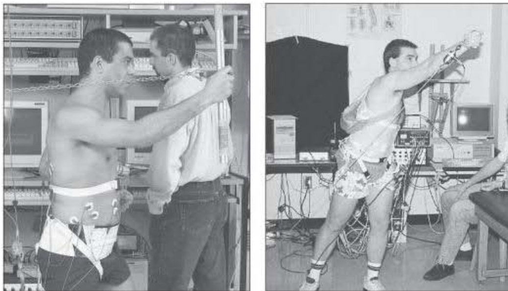
Figure 2.3 In this historical photo on the right, an instrumented subject simulates the complex three-dimensional task of tossing an object. The instrumentation includes three-dimensional video to capture body segment kinematics, a recording of the three-dimensional force vector applied to the hand, a 3-SPACE electromagnetic device to record isolated three-dimensional lumbar motion and assist in partitioning the passive tissue forces, and 16 channels of EMG electrodes to capture muscle activation patterns. A more modern data collection is shown on the left.
