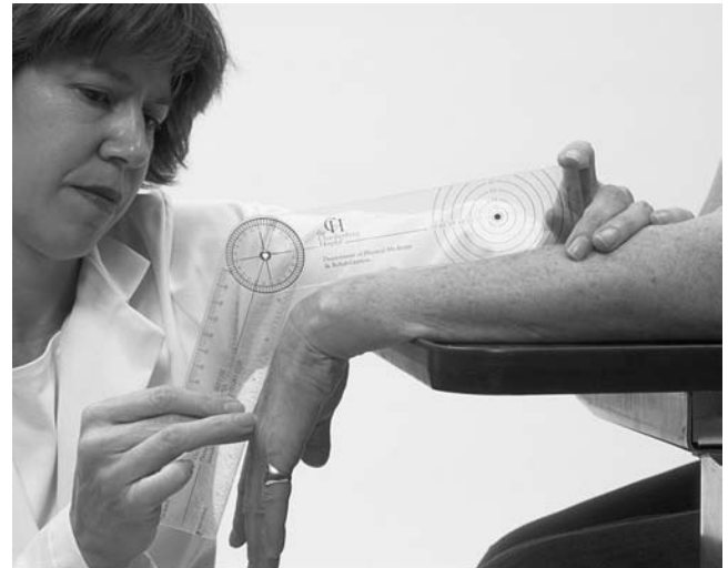
Figure 7.7: A single-axis goniometer to measure joint motion. The single-axis goniometer measures the angular position of a joint.
