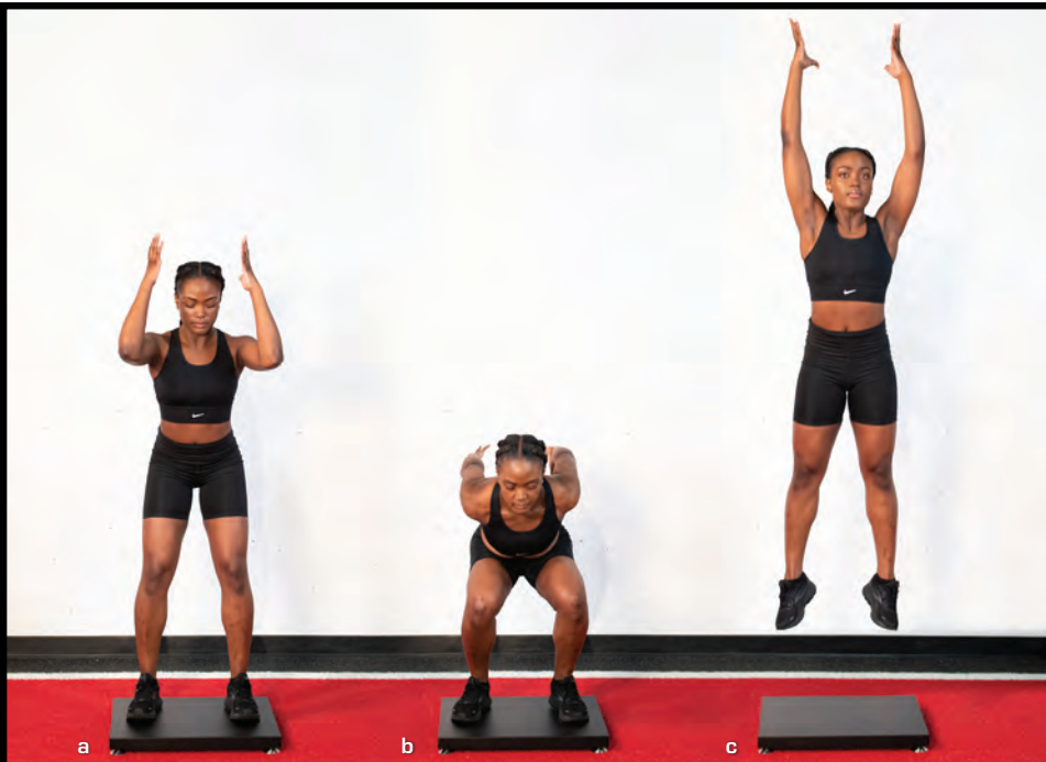
FIGURE 5.1 Sparta Science's platform provides a three-dimensional measurement of the three variables of a vertical jump—load, explode, and drive—which can be used to identify deficiencies and imbalances that affect both injury resilience and performance.
