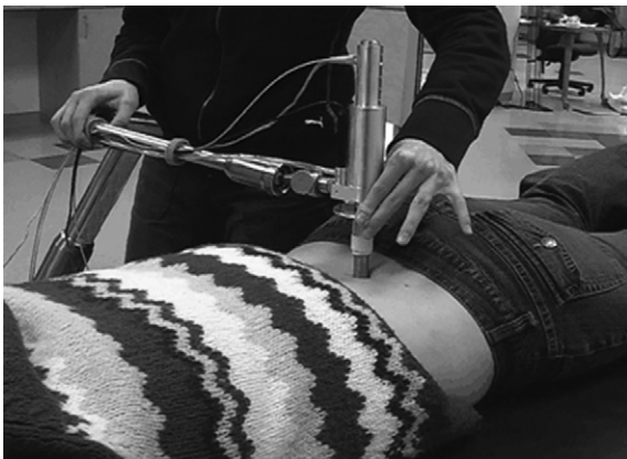
Figure 4.4 Indentation loading applied to the human spine with concurrent quantification of soft tissue deformation and vertebral displacement via onboard ultrasound.
